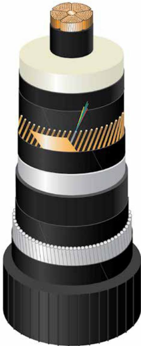
In addition, to ensure the sealing, lead sheath may be used. When this occurs, the cable will have the "K"-index. The lead sheath do not only ensure the sealing but also can replace, partially or in full, the screen transmitting short-circuit currents.
